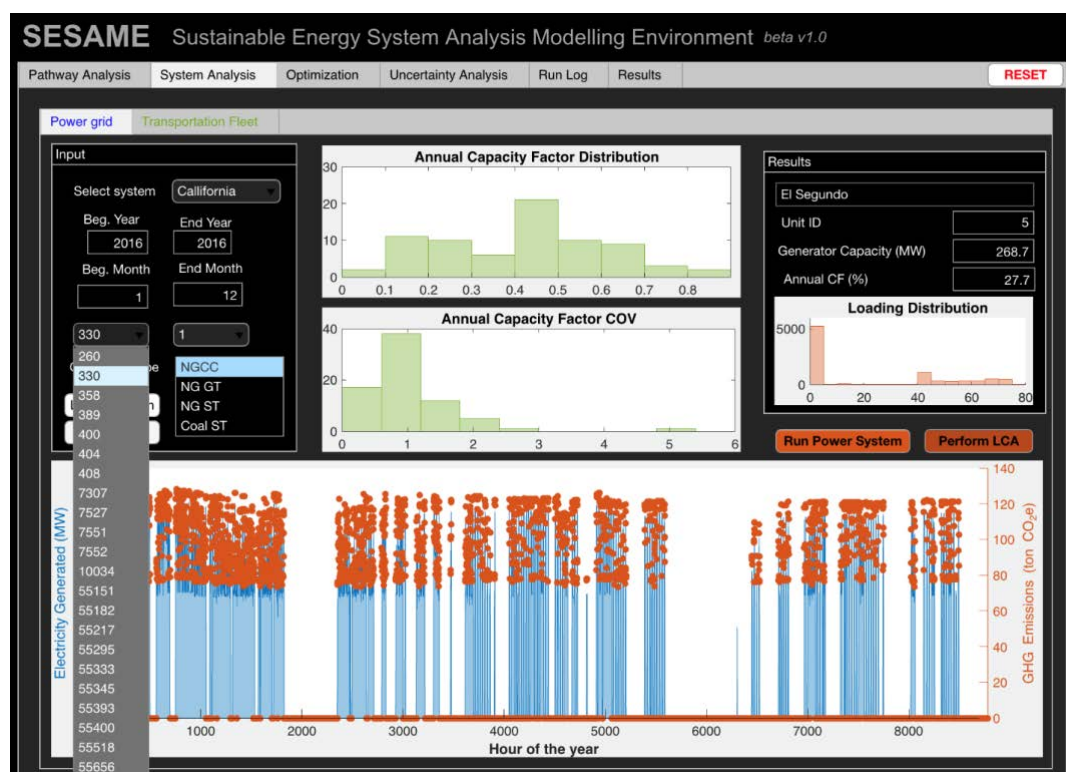
Figure 7 LCA Results at hourly resolution from El Segundo combined cycle power plant unit 5 is estimated using SESAME's power system database. The analysis is performed via the Power Grid Systems Analysis tab of the user interface.
